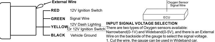
2. Connect the wire, the gauge can be used in Wideballd car.
