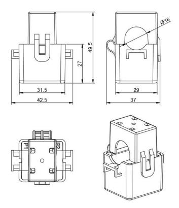
Note: The secondary signal output line is black and white twisted pair, white is S1, black is S2, and the line length is  $2m \pm 10cm$ .
