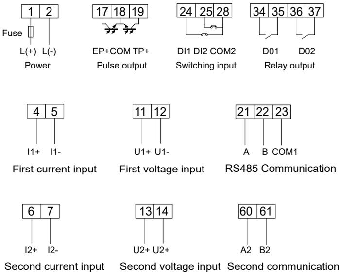
Note: The second DC input channel and DI and DO functions are optional.
