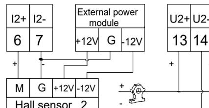
Note: 1. When current shunt is connected to the negative, set the
