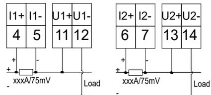
Current shunt connected to the negative
