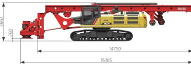
Efficient construction: The most preferred model in civil construction, with fast construction speed and large capacity; adopting the sixthgeneration new material 445 Kelly bar, integrated locking device, drilling capacity increased by 25%, suitable for drilling in multiple strata.
