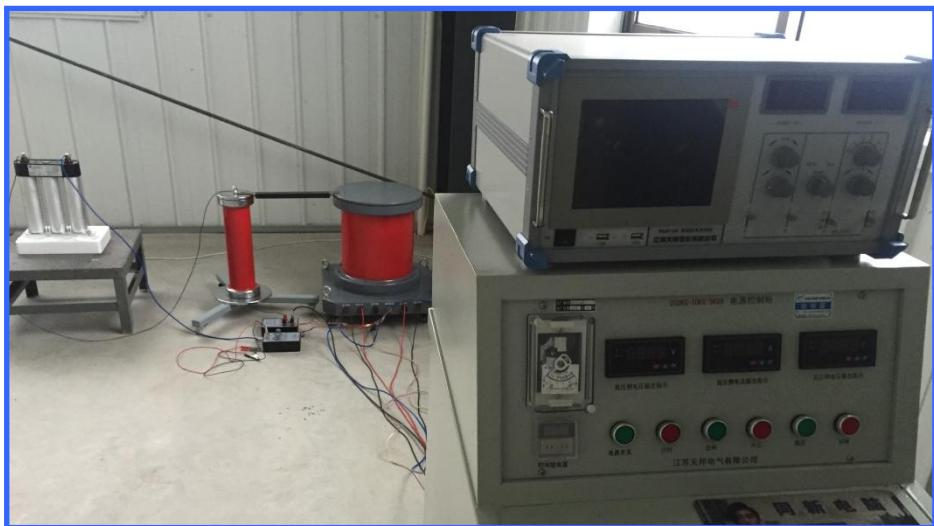
直流充放电设备 Charge and discharge device
