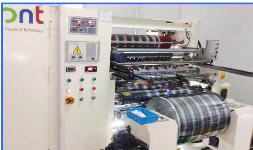
韩国产卷绕机 Winding machine from Korea
