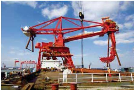
The capacity is 1000-4500t/h. Applicable to the vessel type of 35000~400000DWT. The higher vessel capacity, the more obvious discharging efficient strength.
