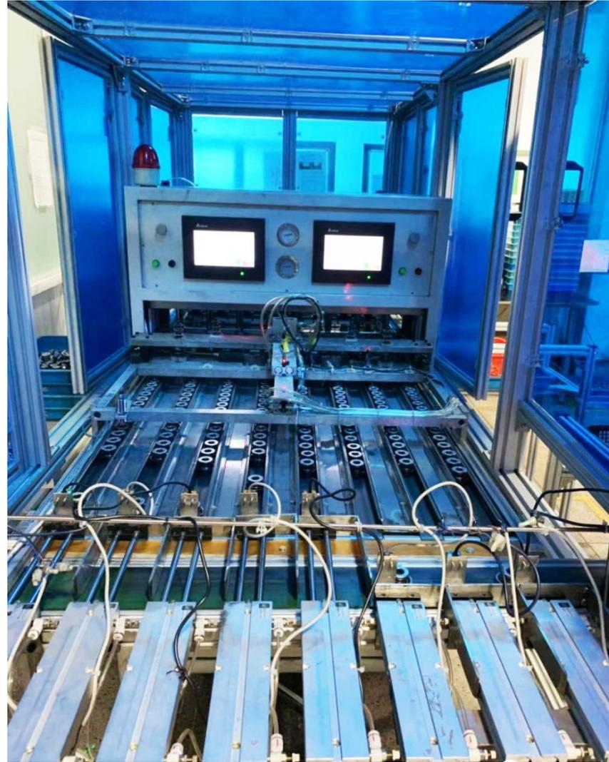
**Automatic Leakage Testing**
