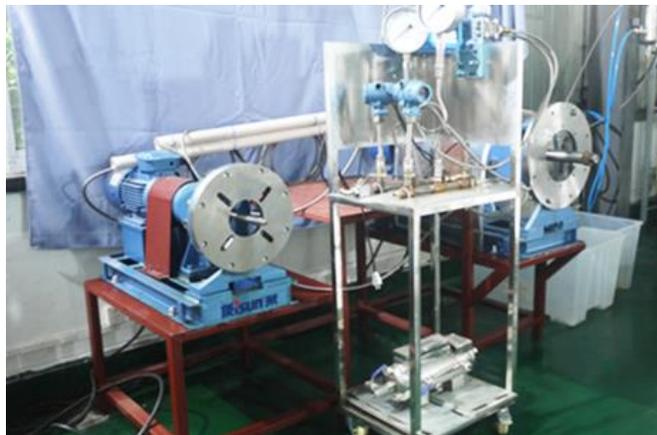
Chemical pumps Rotating Life Test Bench
