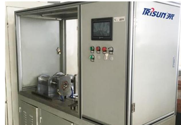
Auto-cooling pump testing system
