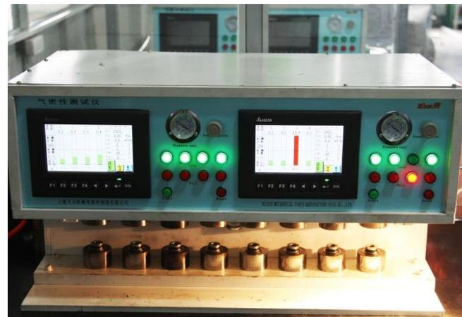
Seal Static leakage testing system
