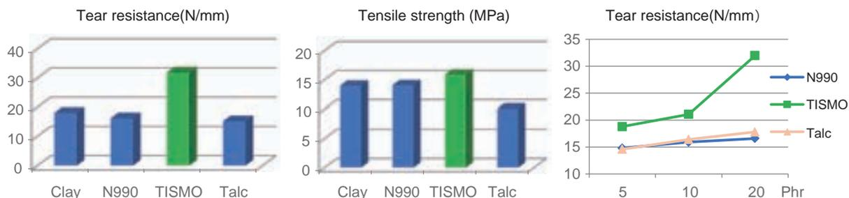
TISMO added by low shear mixing process, improves fluoroelastomer's high temperature tear resistance and tensile strength, along with the thermal stability. As the addition amount of TISMO increases, tear resistance and thermal resistance increase significantly. Recommended adding amount is 5~25phr. TISMO has superior friction feature, especially suitable for products like oil sealings, which requires high tear resistance and thermal stability.
