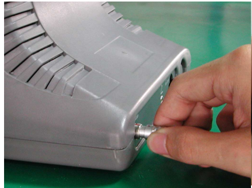
Pic.3 Pull and plug the probe
