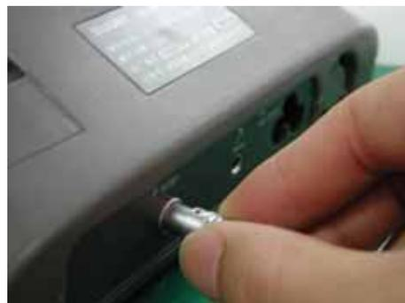
Pic.3 Plug and pull the probe
