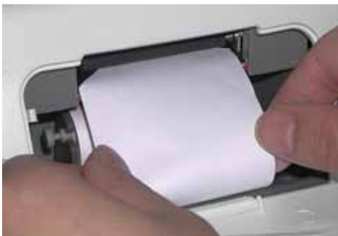
Pic.17 Press S/L to roller paper
