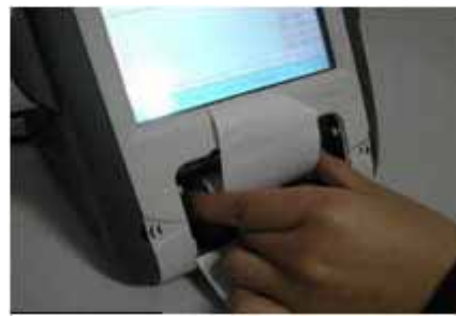
Pic.16 Refill roller, see paper end
